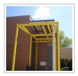
An I-beam monorail system with curves and switches was installed when the room was built in the late 1960's. The hoist was replaced 10 years ago and powered by electrification bar. Maintenance was required frequently and was getting progressively worse. For the final six months that the system was used, it was down an average of twice per week.
