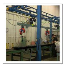
The 28 foot long pieces of track are rolled out on a conveyor for one side to be assembled. The 1304lb track then needs to be lifted, flipped over, and set back down on the conveyor for the underside to be assembled. When designing this new work cell, safety of the workers was a very big concern. The company researched several options and discovered that the Gorbel solution was not only simpler and safer, but it was one third the cost of other designs.
