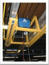
A G-Force® Intelligent Lifting Device with Float Mode was demonstrated to the customer. They realized that the float mode not only gave them the speed control they were looking for, but also provided an easier way to line up the rolls to the donut holes on the machine by using their hands to control the load.
