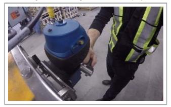
coating line using the Gorbel G-Force®. The bin foundation is lifted from a stack and then hung on hooks suspending the product as it goes through the line. At the end of the line the product is removed from the hooks and stacked using the same G-Force® handling device.
