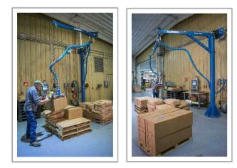
A Gorbel Easy Arm® Intelligent Lifting Device was the solution. The technology enables the operator to lift and maneuver naturally, as if the device were an extension of their own arm. It has given them the ability, "to be able to lift it with the fingertip". They are very impressed with the flexibility the system offers. "It allows a very fluid and ease of motion to move boxes and bags with." They feel it is a great piece of equipment that will keep their older employees working safely.
