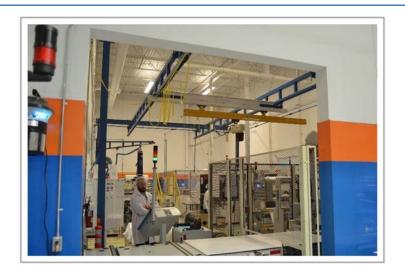
The floor area was very congested and there was an overhead venting obstruction associated with the new machine installation that could not easily be modified. A standard Bridge Crane layout would not work as a lifting solution because of this obstruction. Consideration was given to using two jib cranes but that idea was disqualified because it would have meant a two-step lifting operation to handle the rolls.
