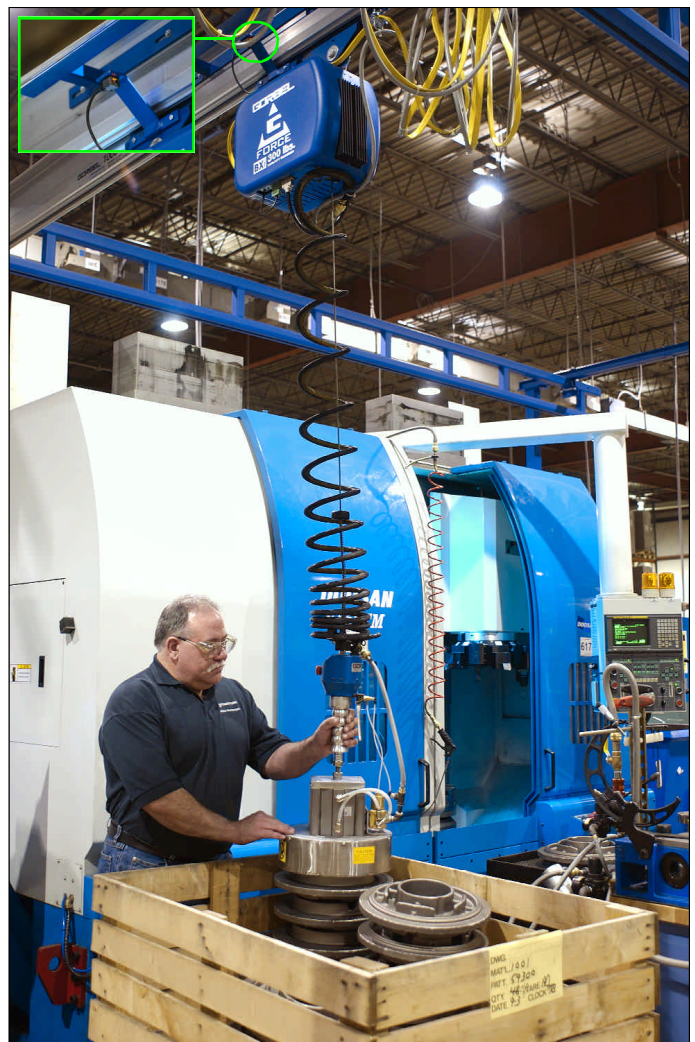
The operator can lift the parts out of the bin at his natural pace. When he enters Zone 2, the sensor shown above reacts to a target mounted above the machine, activating pre-programmed virtual limits and speed reduction points. When activated, the G-Force™ automatically shifts into a slower speed to prevent the operator from slamming the part into the chuck.
