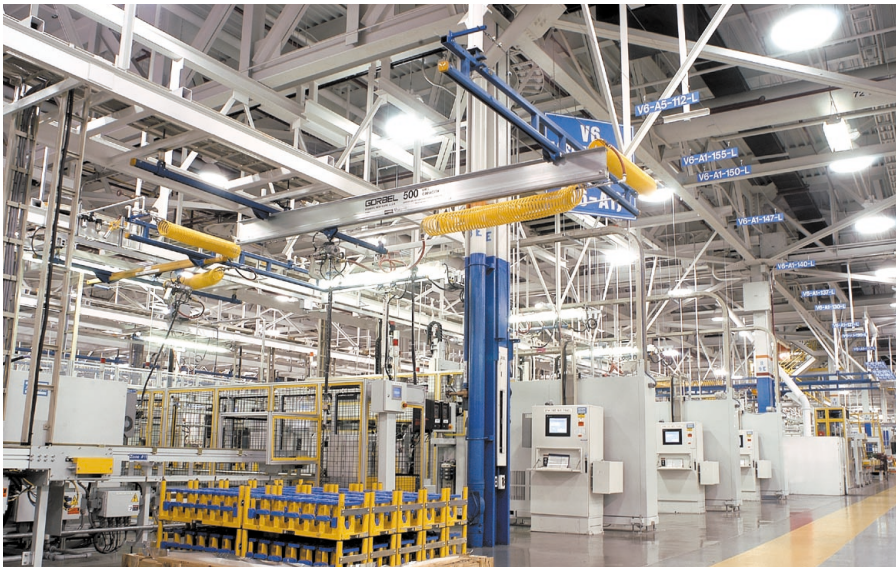
A GM requirement was that the Gorbel cranes be rigid, so as to deliver predictable motion and force.
