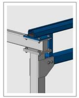
Gorbel track. All rails were inverted to minimize dust and particles from falling on the equipment below. The post to header/rail attachments were custom engineered to maximize head room. All motions are set to super slow speeds to reduce the risk of damaging materials and equipment.
