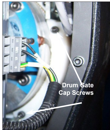
Diagram R. Remove two M6 socket head cap screws from the drum gates.
