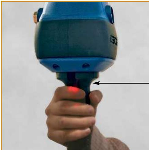
Use a gentle puff of compressed air or a soft cloth to clean the sensor. Do not apply any pressure to the lens or do anything that may scratch it.
