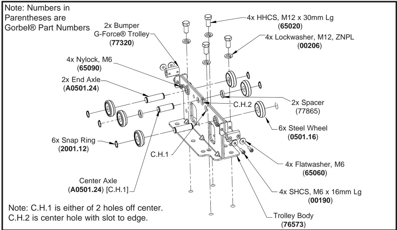
Trolley Components for 500 Series Steel Track.
