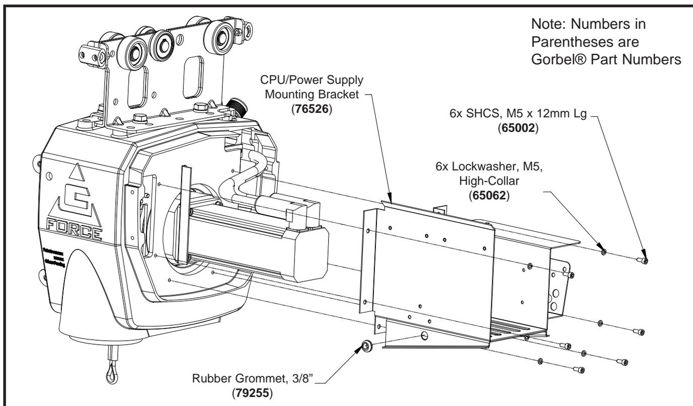
**Diagram 10.** CPU/Power Supply Mounting Bracket Removal and Replacement.
