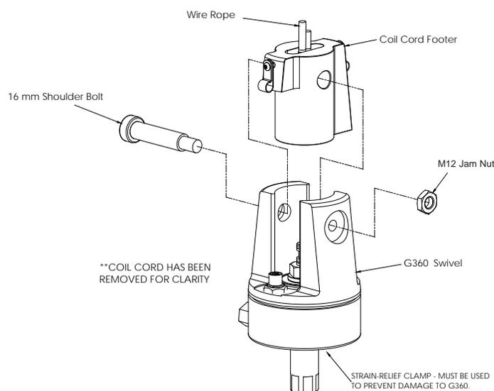
**Diagram 5B.** G360™, Shoulder Bolt and Coil Cord.
