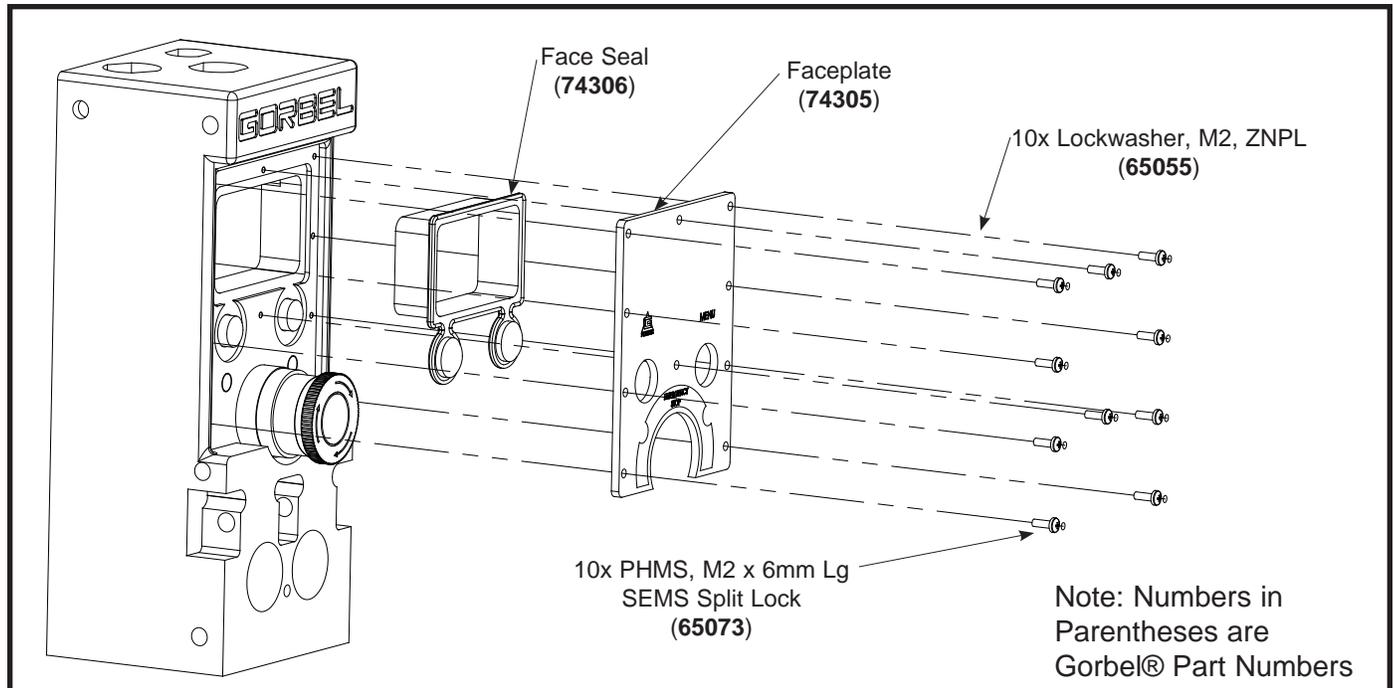
**Diagram 9.** Faceplate and Face Seal Removal and Replacement.
