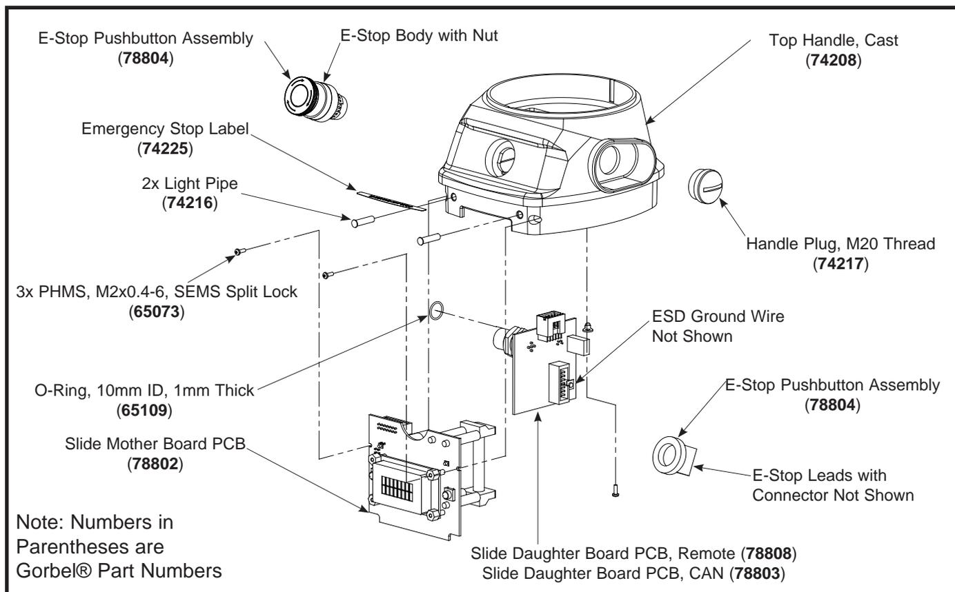
Diagram 4A. Housing Sub-Assembly Assembly and Disassembly.
