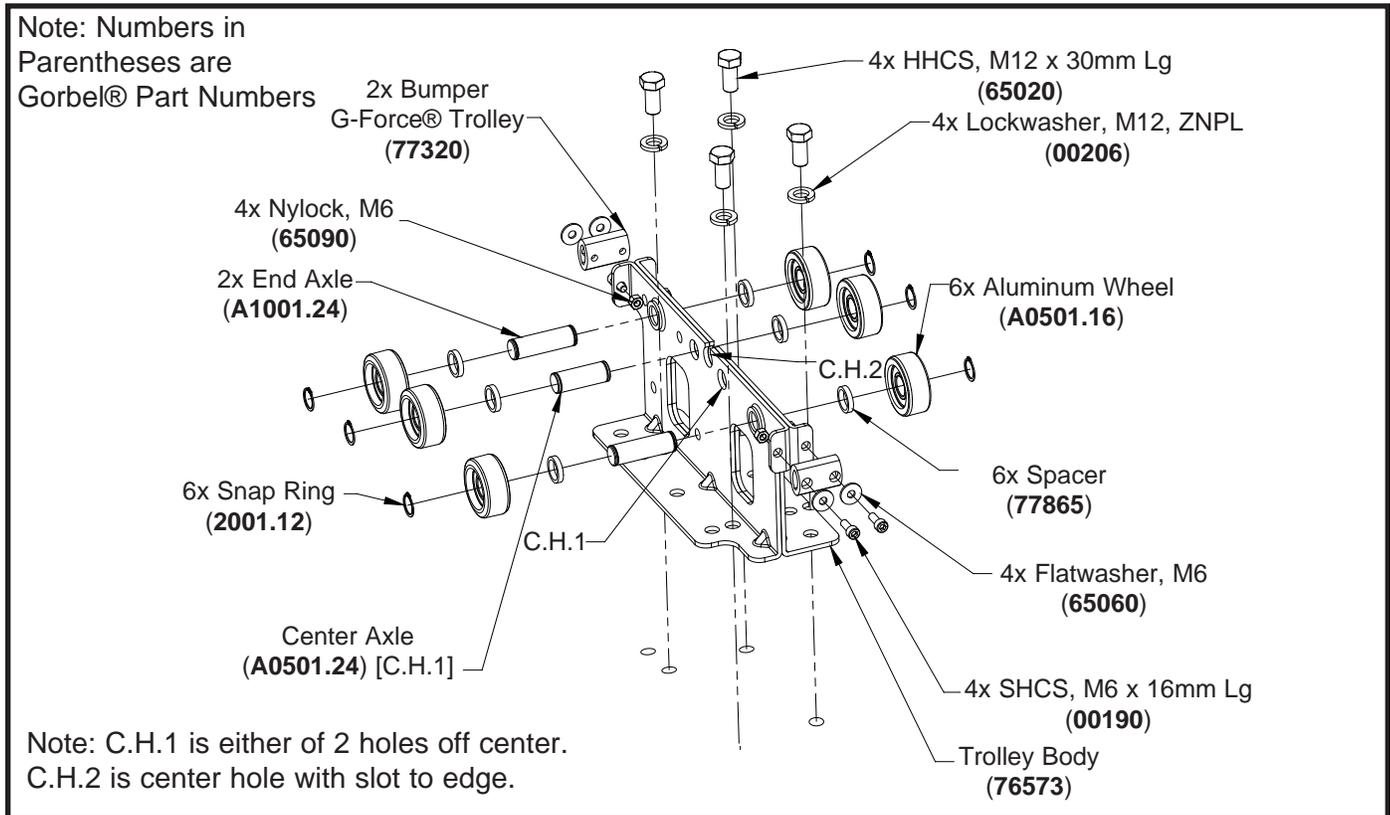
Trolley Components for 500 Series Aluminum Track.
