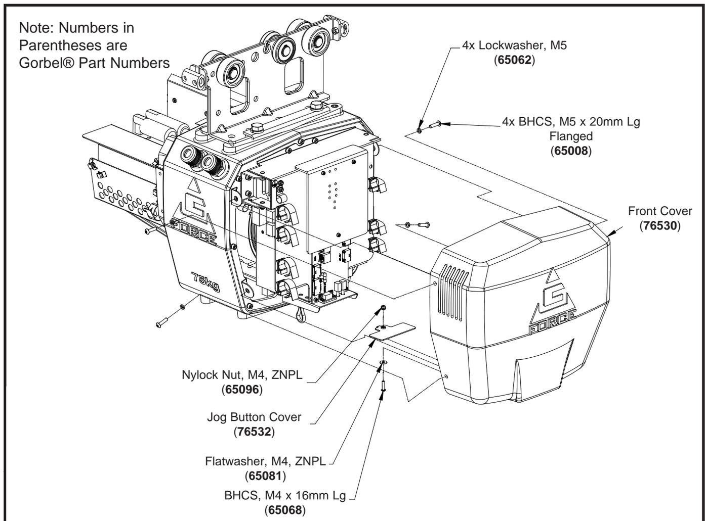
Diagram 1. Front Cover Removal and Replacement.
