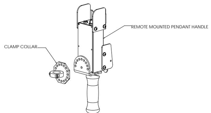
**Diagram 5I.** Remote Mounted Pendant Handle with Collar Clamp Mounting Bracket (Option).
