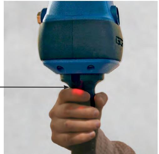
8. **Handle I/O Connections (both handles):** Check connections at handle (if equipped). Wipe off any oil or other contamination from either Handle at this time. Clean the LCD screen as well.
