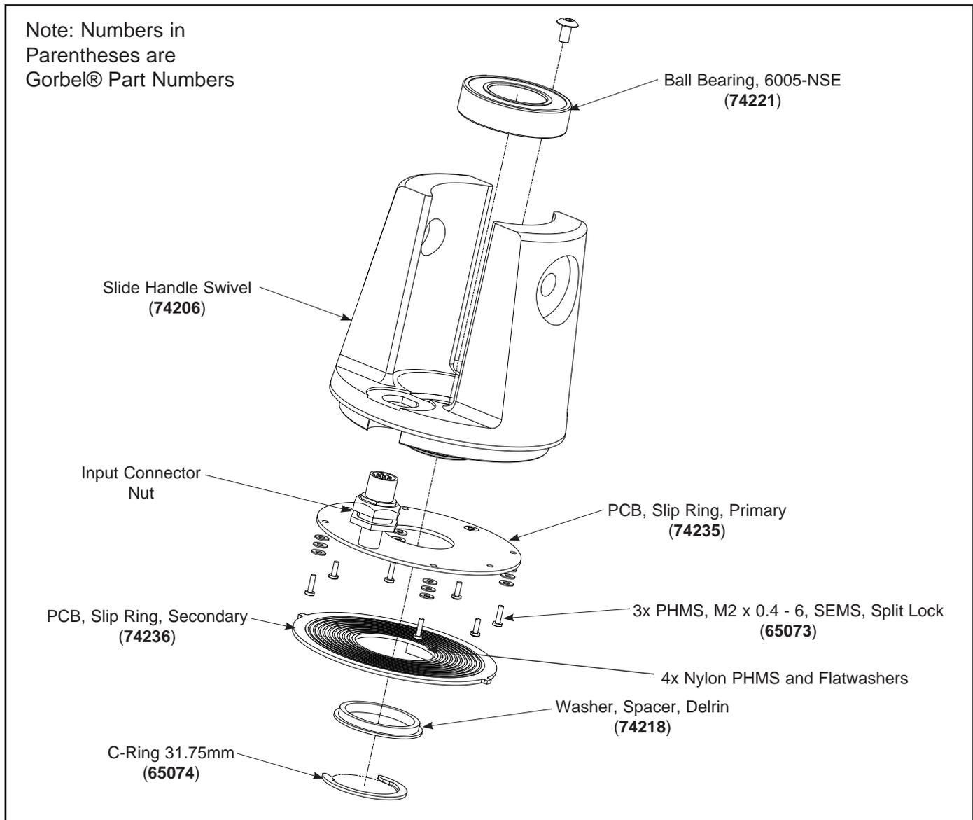
Diagram 2. Swivel Sub Assembly Disassembly and Reassembly.
