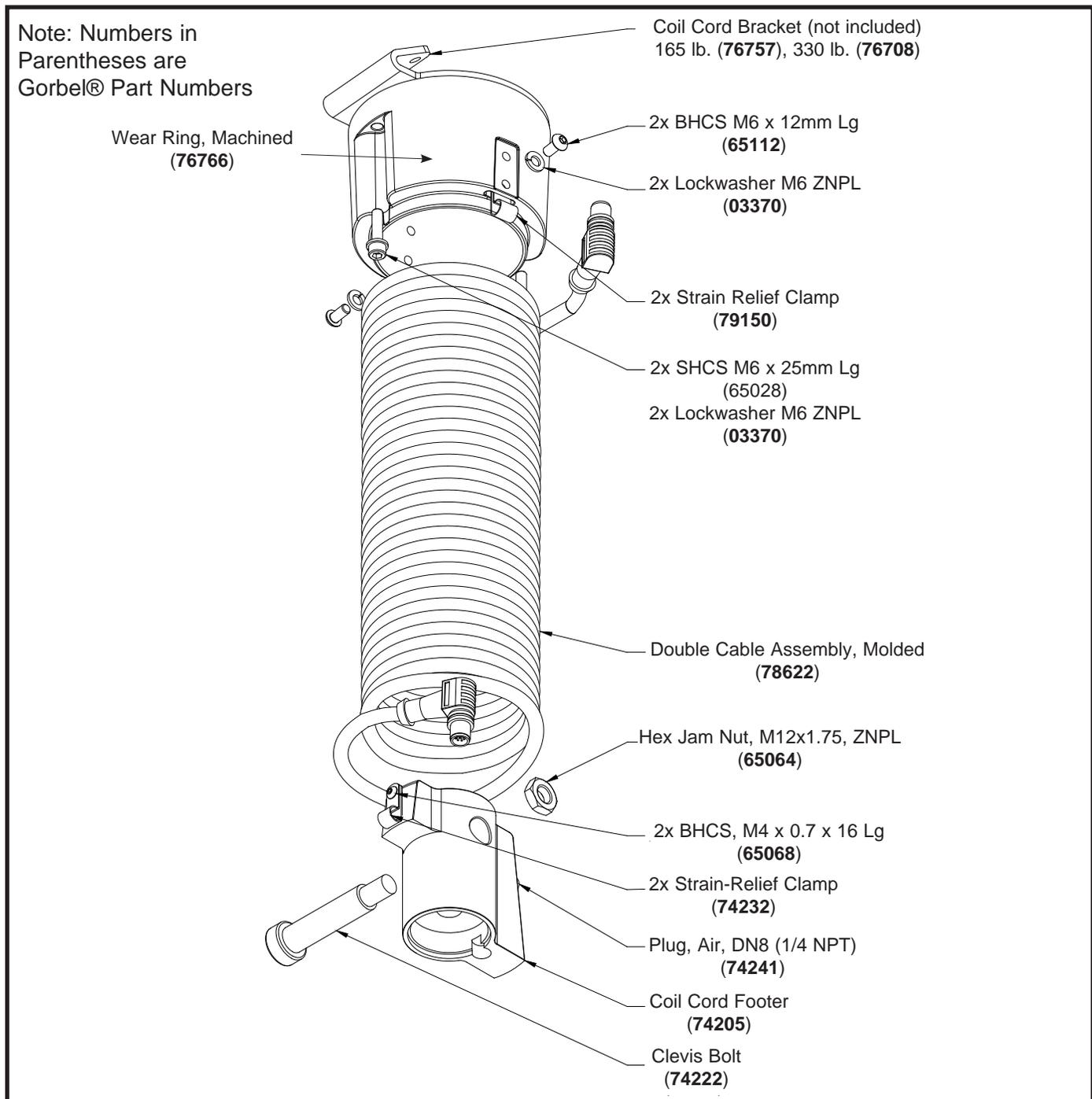
Diagram 4. 165 lb. (75 kg) and 330 lb. (150 kg) Double Length Coil Cord Assembly.
