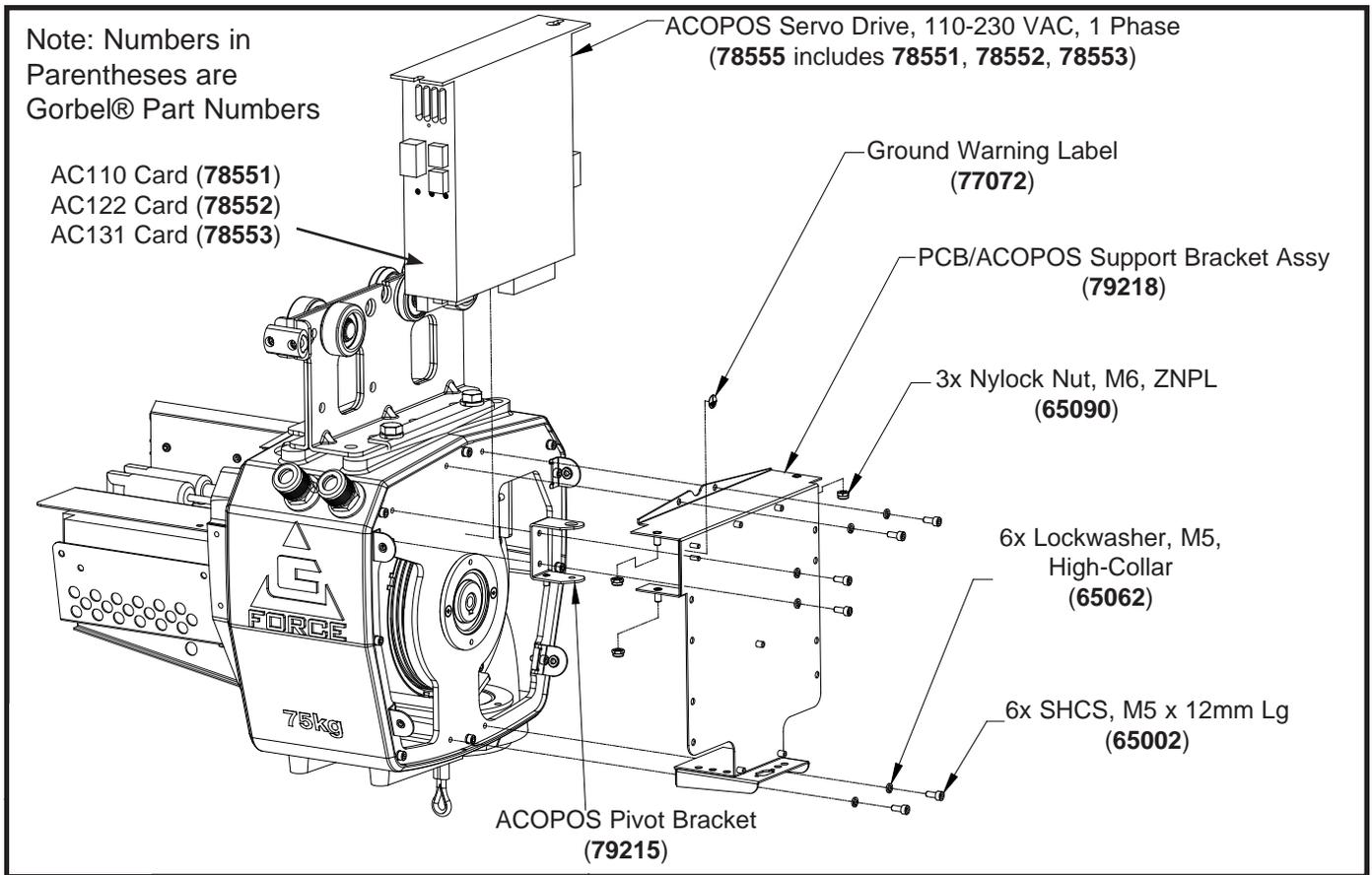
Diagram 7. ACOPOS and Support Bracket Removal and Replacement.
