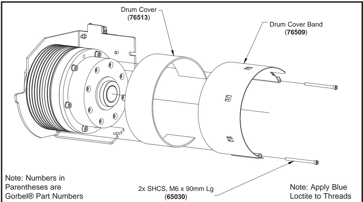
Diagram 15B. 660 lb. (300 kg) Drum Cover and Band Removal and Replacement.
