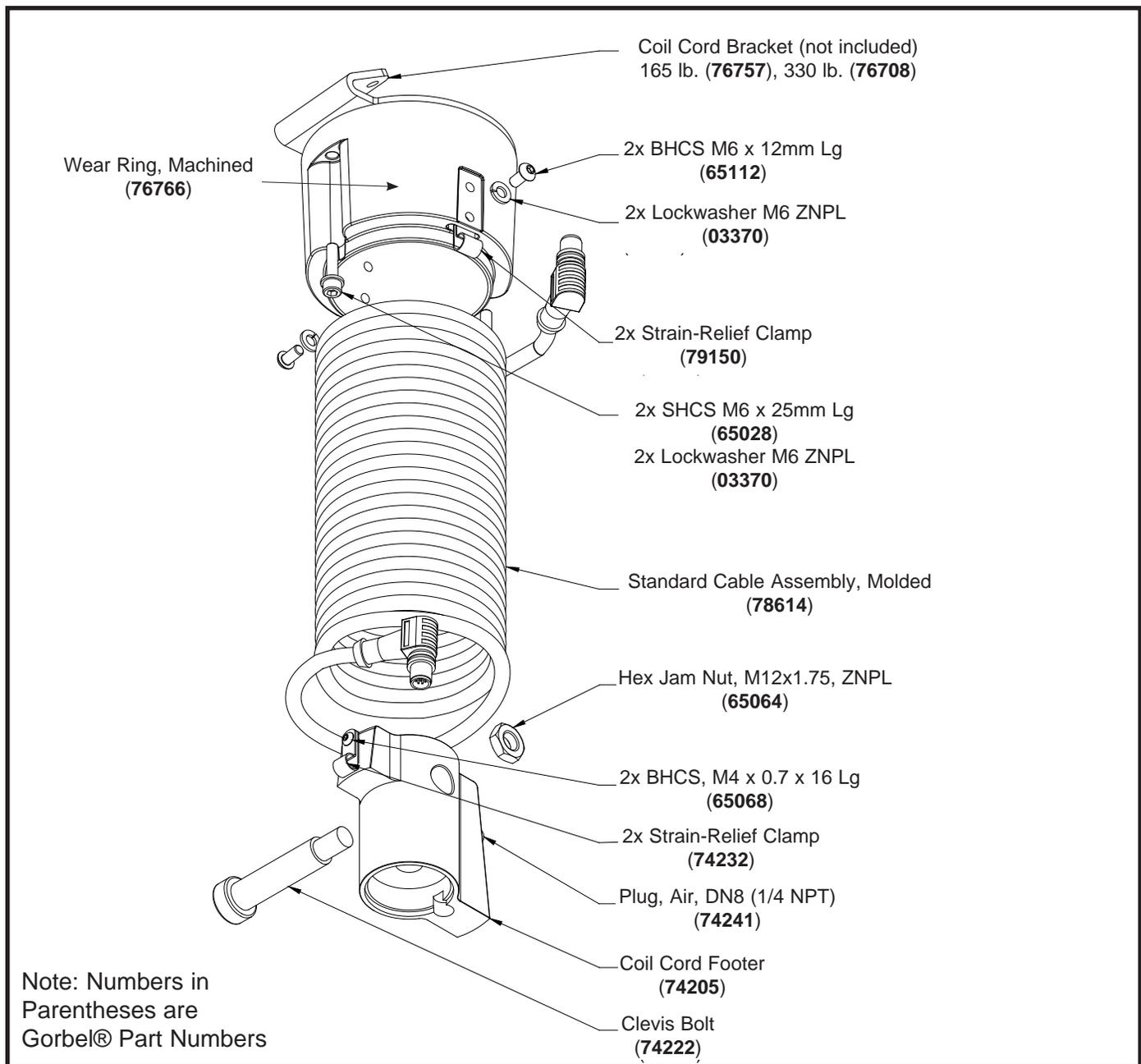
Diagram 2. 165 lb. (75 kg) and 330 lb. (150 kg) Standard Length Coil Cord Assembly.
