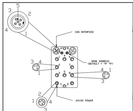
Diagram 5. Handle Input/Output Block.
