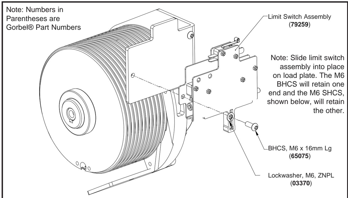
**Diagram 16A.** 165 lb. (75 kg) and 330 lb. (150 kg) Limit Switch Assembly Removal and Replacement.
