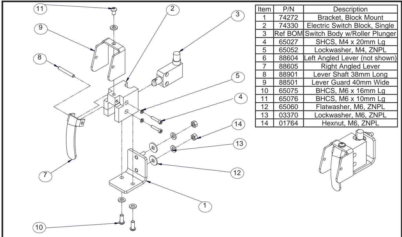
Single Electric Switch Assembly for Slide Handle.
