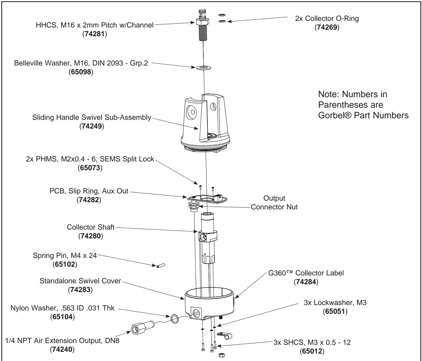
Diagram 1A. G360™ with Air Assembly and Disassembly.
