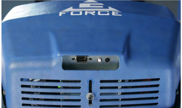
7. **Operator Present Sensor (sliding handle only):** Use a gentle puff of compressed air or a soft cloth to clean the sensor. Do not apply any pressure to the lens or do anything that may scratch it.
