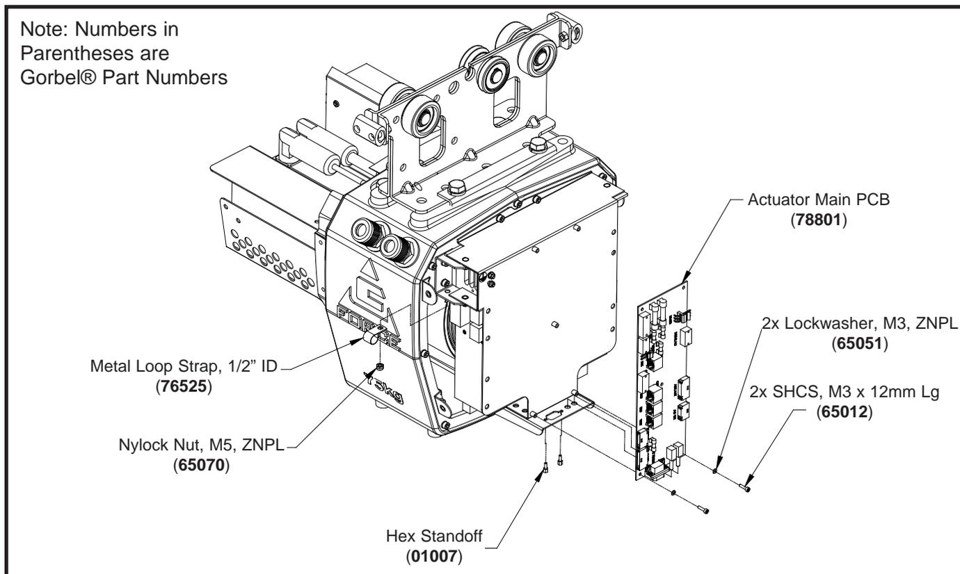
Diagram 5. Main PCB Removal and Replacement.
