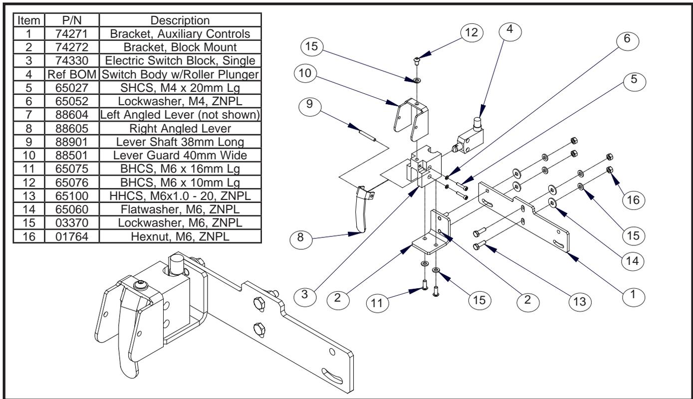
Auxiliary Electric Switch with Bracket.
