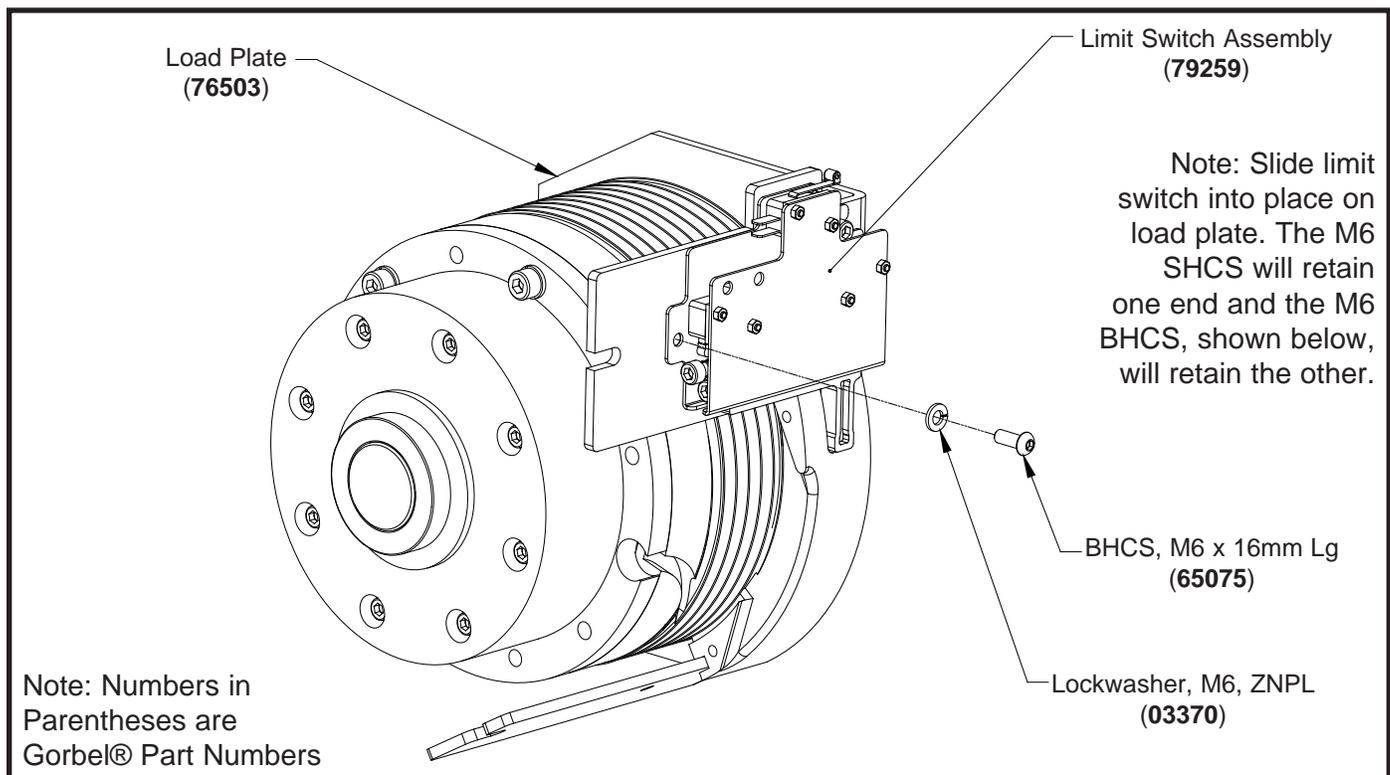
**Diagram 16B.** 660 lb. (300 kg) Limit Switch Assembly Removal and Replacement.
