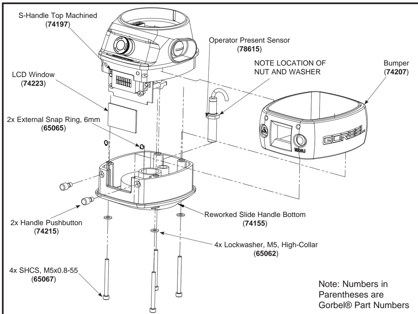
Diagram 2. Housing Sub-Assembly Removal and Replacement.
