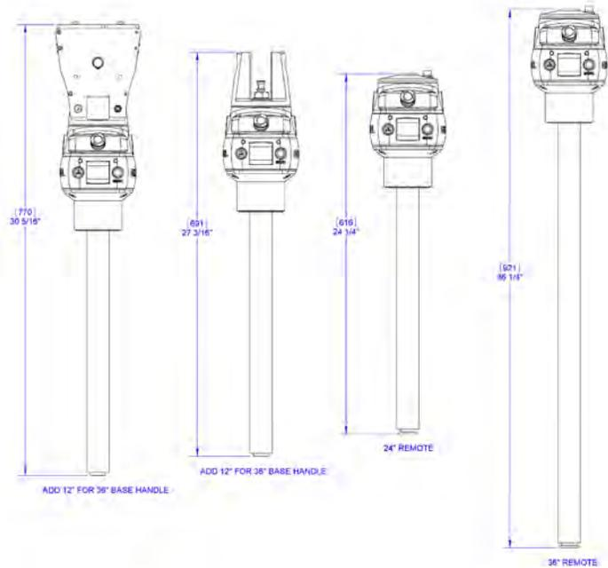
**Diagram 5M.** Force Sensing Slide Handle bracket sizes.
