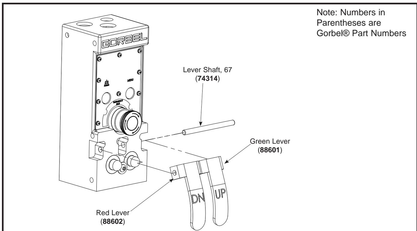
**Diagram 4. Lever Removal and Replacement.**
