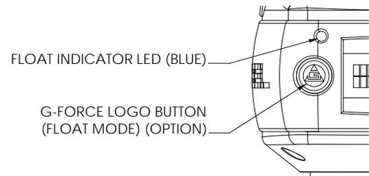
**Diagram 8A.** Float Mode Button - Slide Handle.
