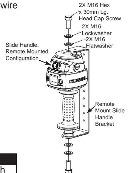
**Diagram 5D.** Remote Mounted Slide Handle, Exploded View.
