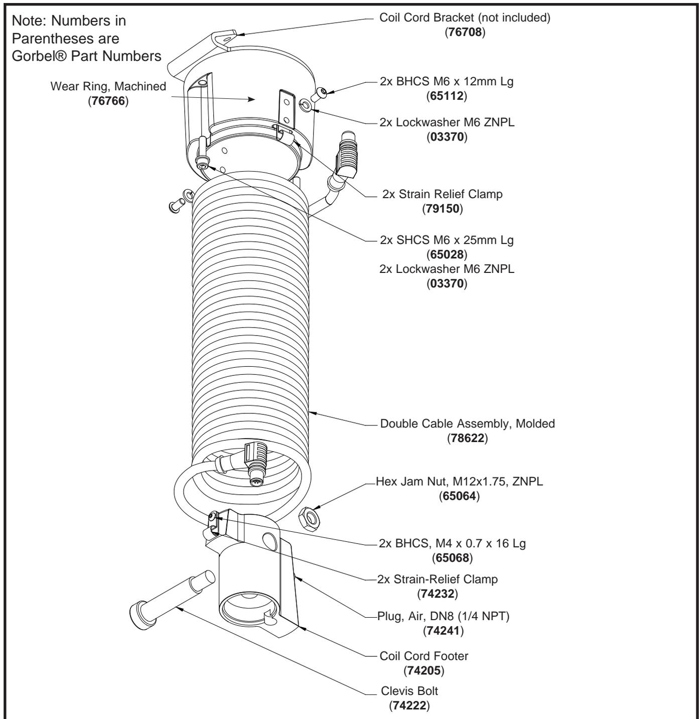
**Diagram 3.** 660 lb. (300 kg) Double Length Coil Cord Assembly.
