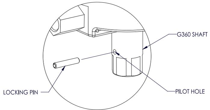
**Diagram 5C.** Tooling Installation.
