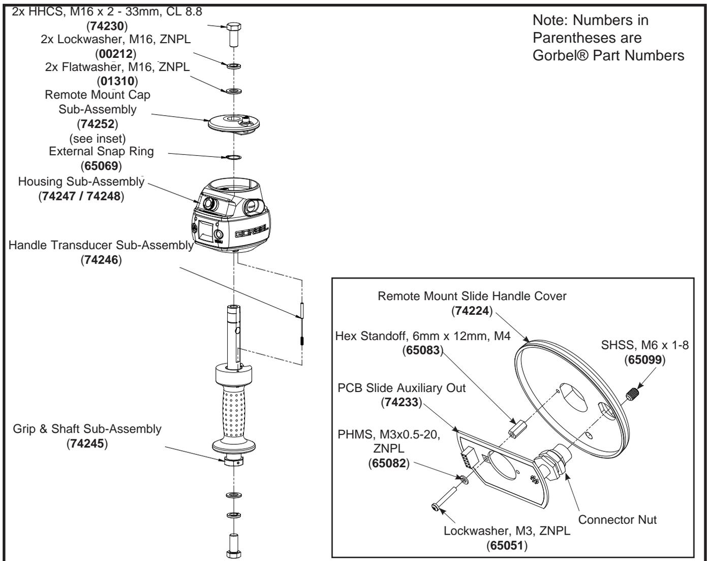
Diagram 2. Remote Mounted Sliding Handle Remote Mount Cap Sub Assembly Removal and Replacement.
