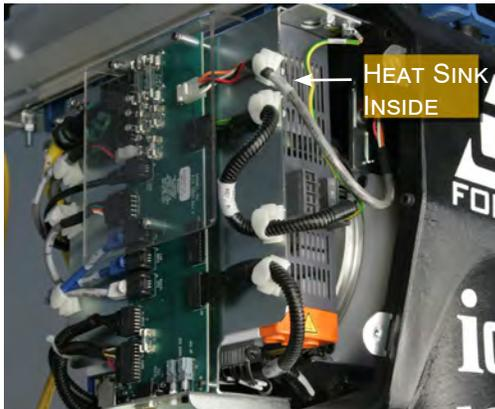
**15. Cooling Fan (if equipped):** Clean this area if it appears to be dirty. Use compressed air and safety glasses.
