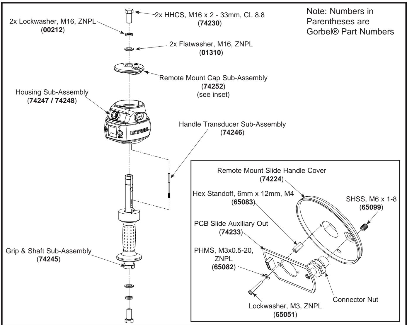
**Diagram 5. Handle Transducer Sub Assembly Removal and Replacement.**
