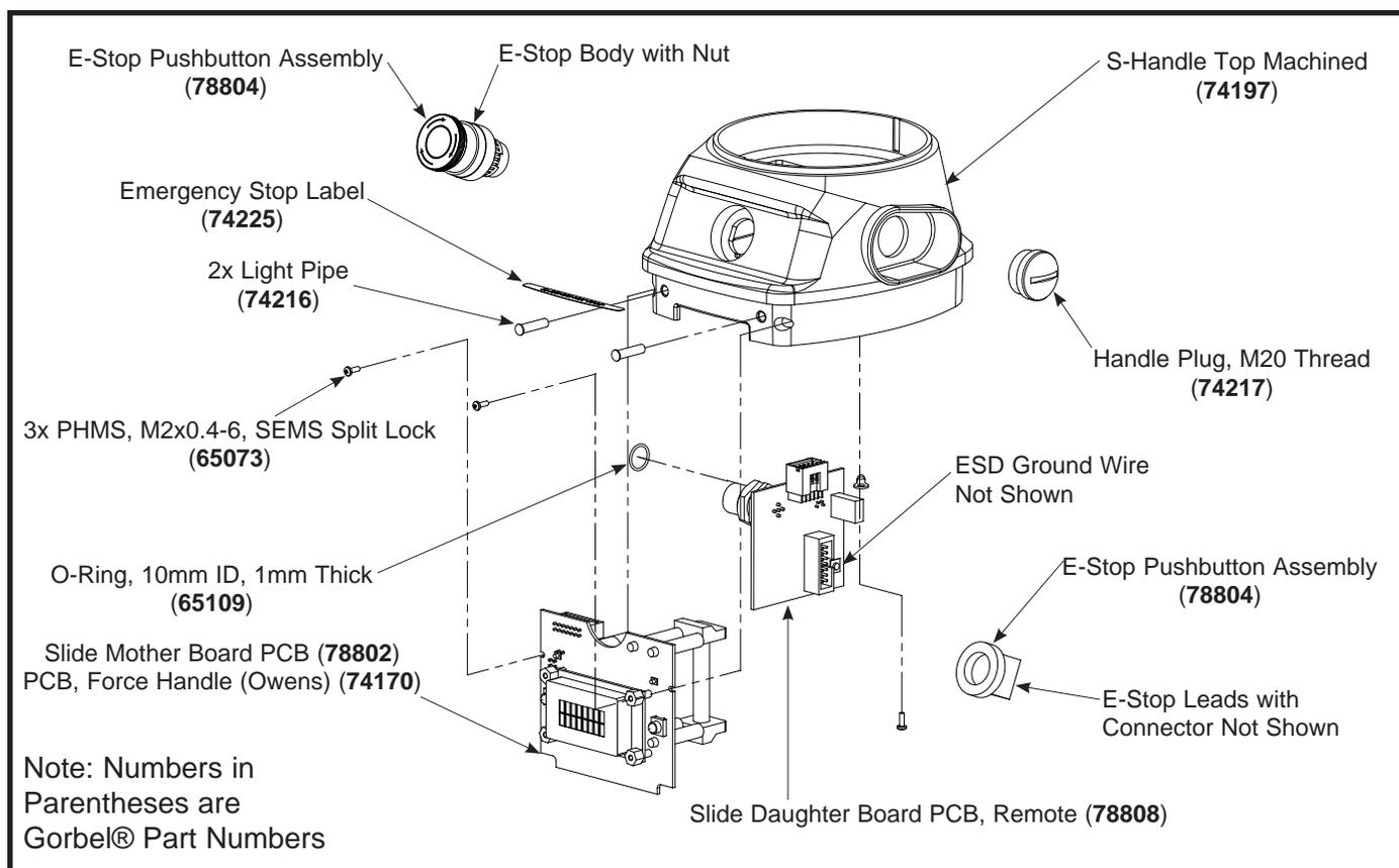
Diagram 3A. Housing Sub-Assembly Assembly and Disassembly.
