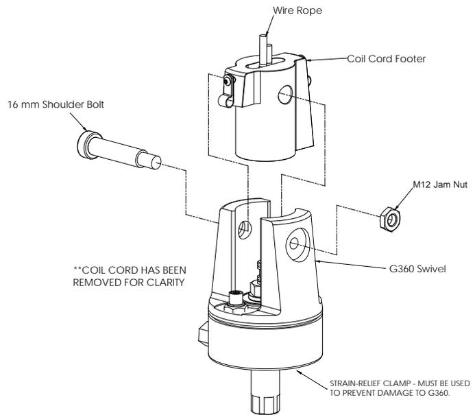
**Diagram 5G.** G360™, Shoulder Bolt and Coil Cord.
