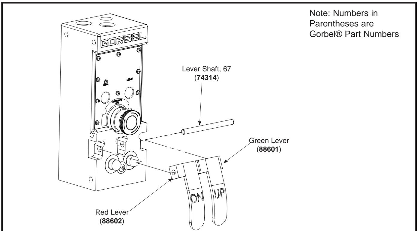
Diagram 3. Lever Shaft Removal and Replacement.
