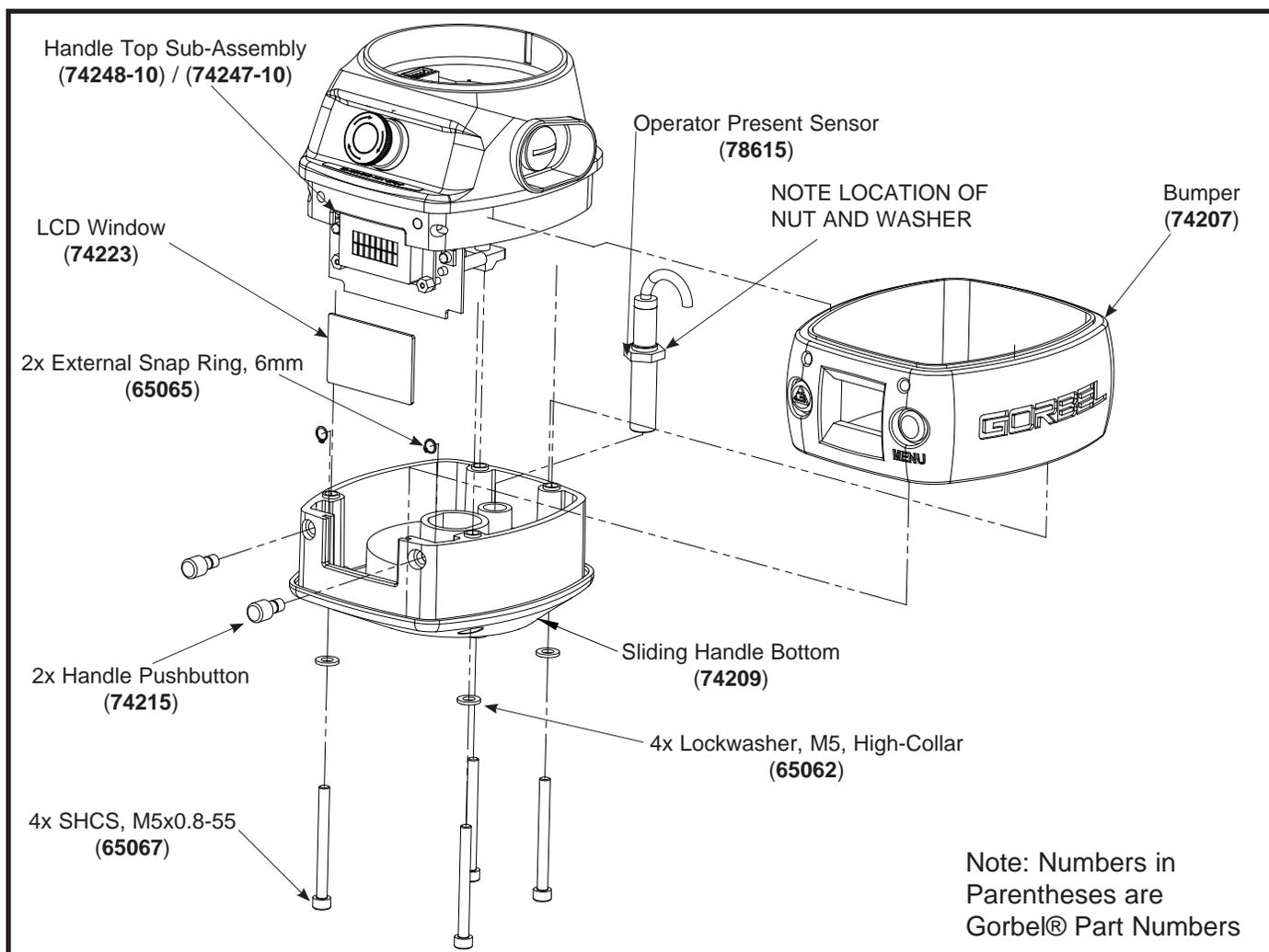
Diagram 3. Housing Sub-Assembly Removal and Replacement.
