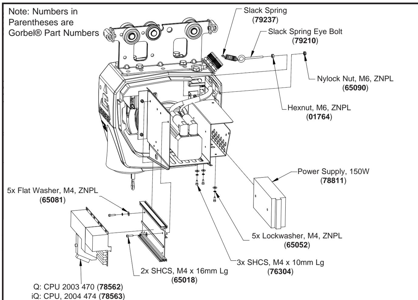
Diagram 8. CPU Assembly Removal and Replacement.
