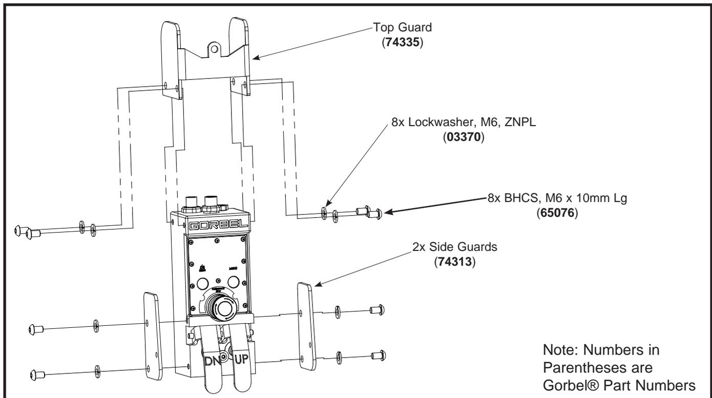
**Diagram 2.** Side Guard Removal and Replacement.
