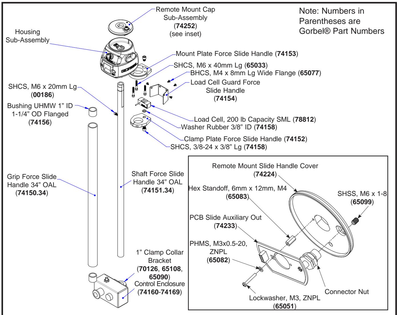
**Diagram 1.** Remote Mounted Force Sensing Sliding Handle Remote Mount Cap Sub Assembly Removal and Replacement.
