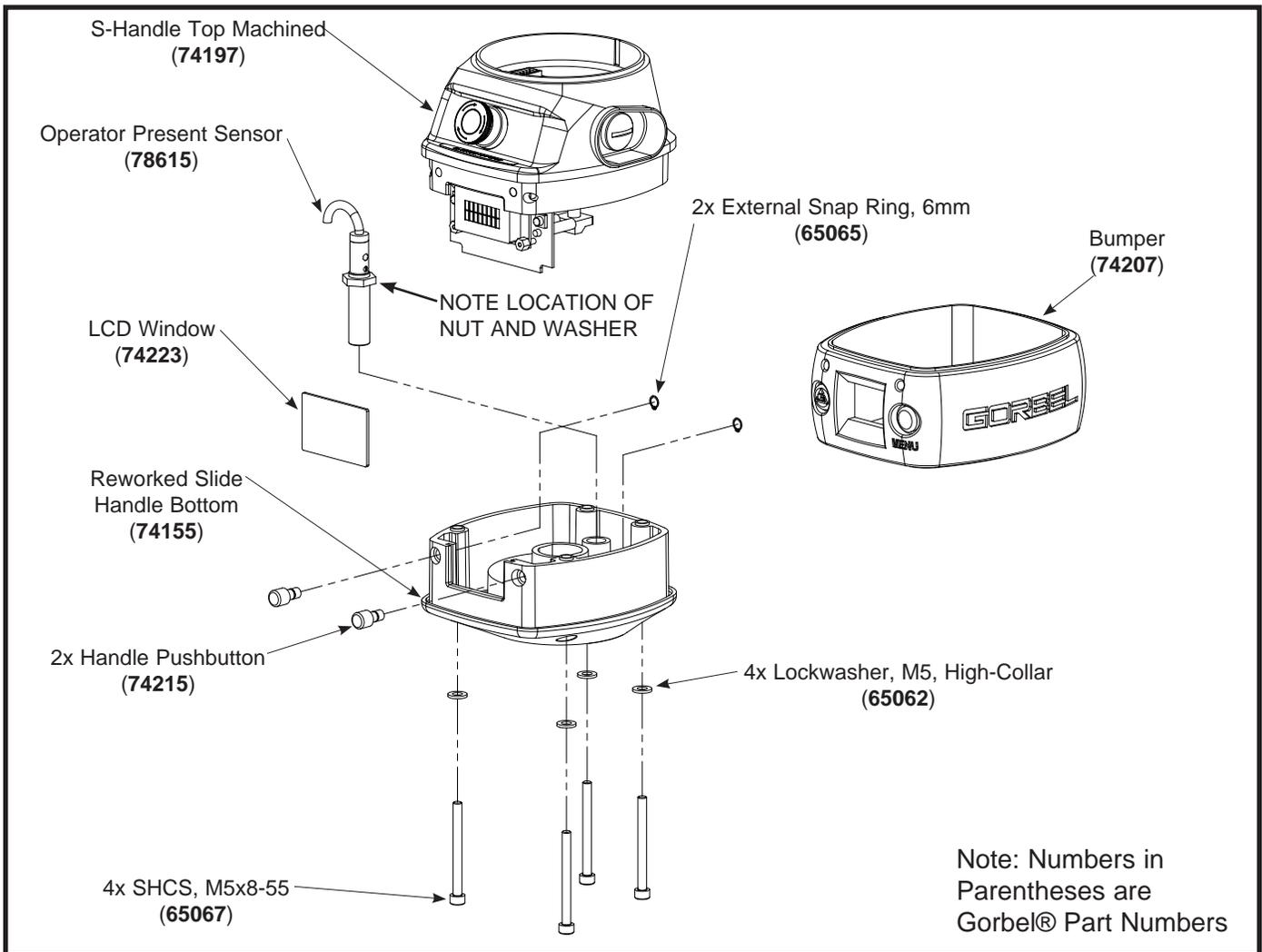
Diagram 3B. Housing Sub-Assembly Assembly and Disassembly.
