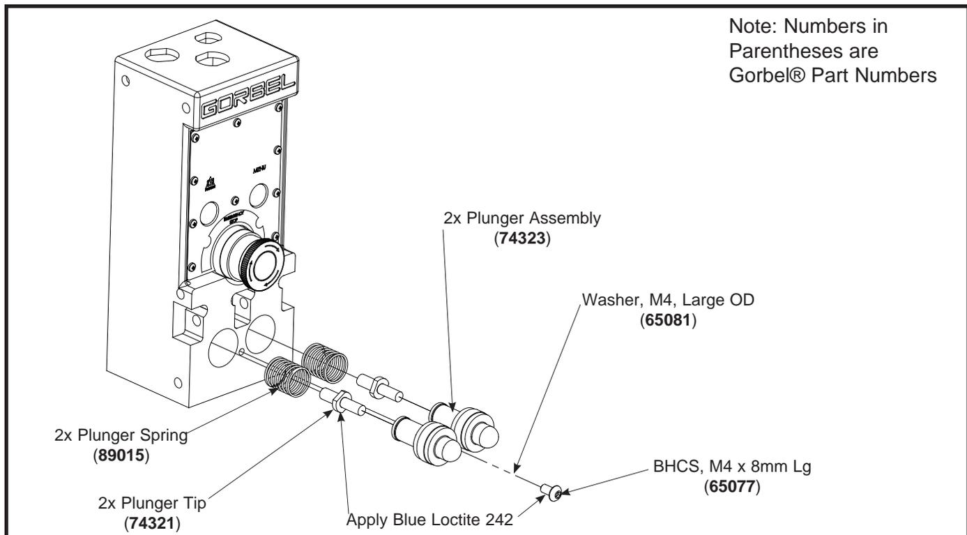
**Diagram 8.** *Plunger Assembly Removal and Replacement.*
