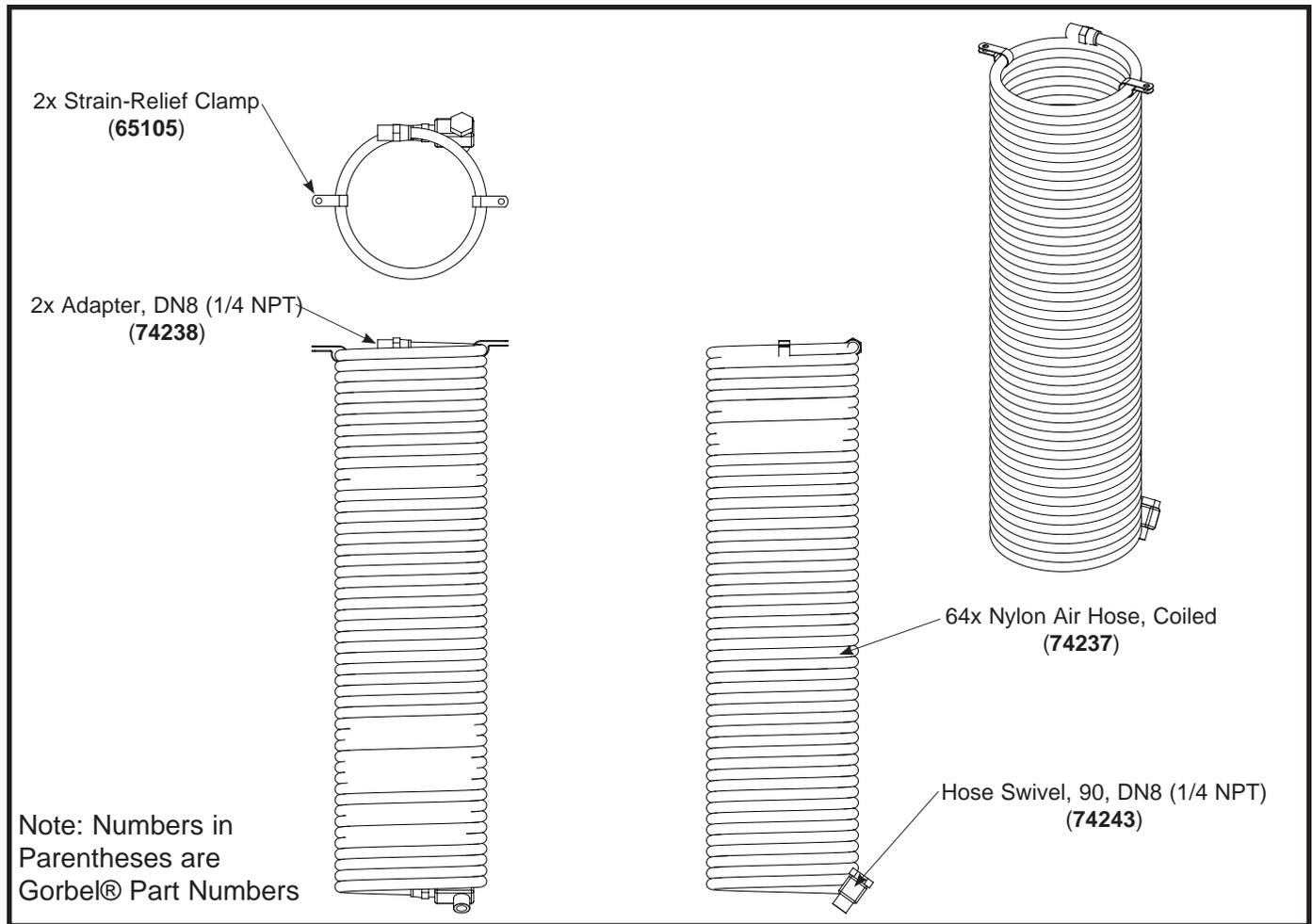
Diagram 6. Extended Length Air Hose Assembly.
