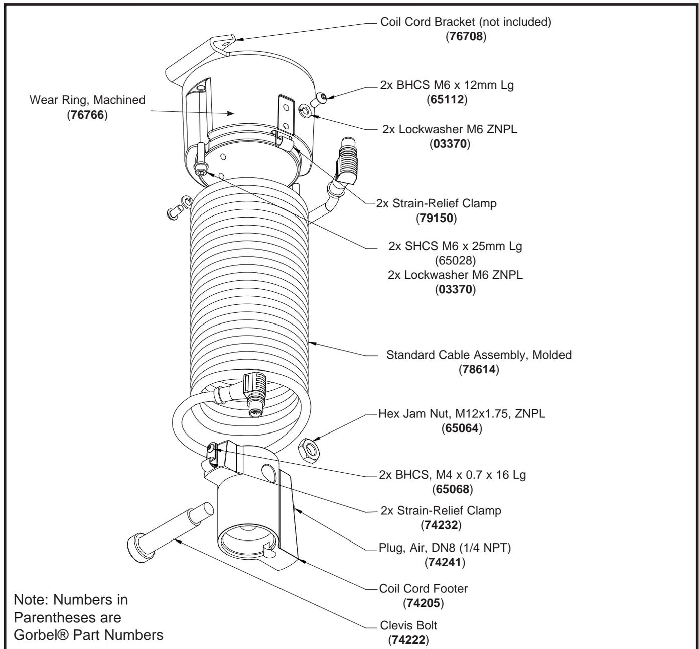
**Diagram 1.** 660 lb. (300 kg) Standard Length Coil Cord Assembly.
