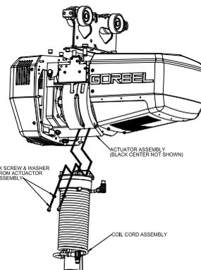
**Diagram 4C.** Coil Cord Assembly Installation at the Actuator.
