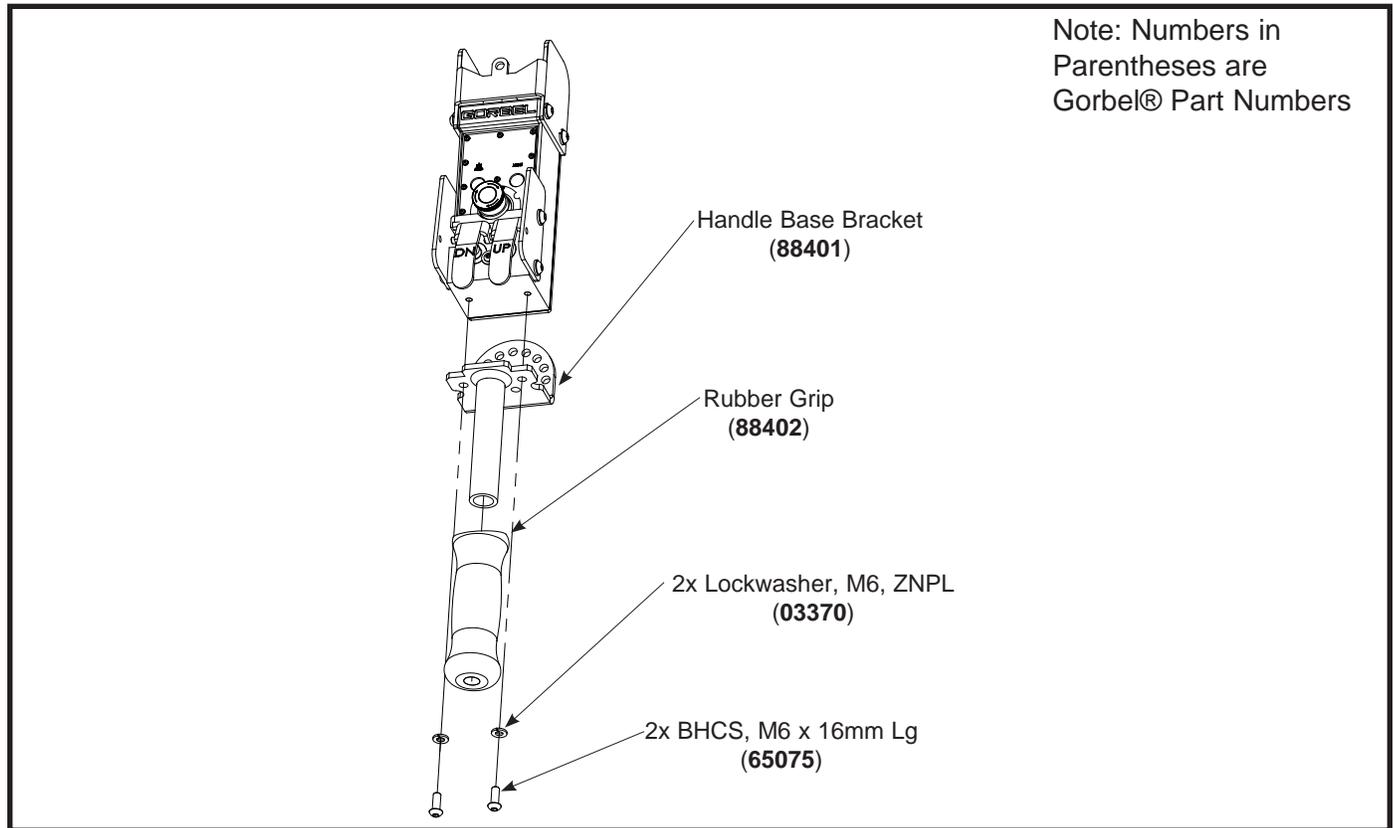
**Diagram 5.** Handle Base Bracket Removal and Replacement.
