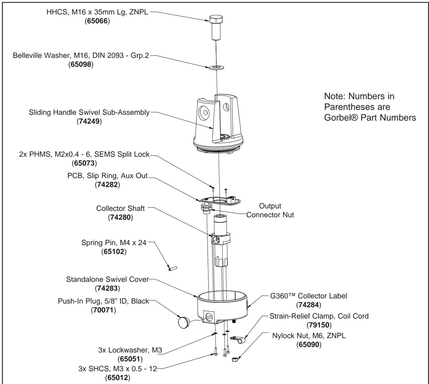
Diagram 1B. Standard G360™ Assembly and Disassembly.
